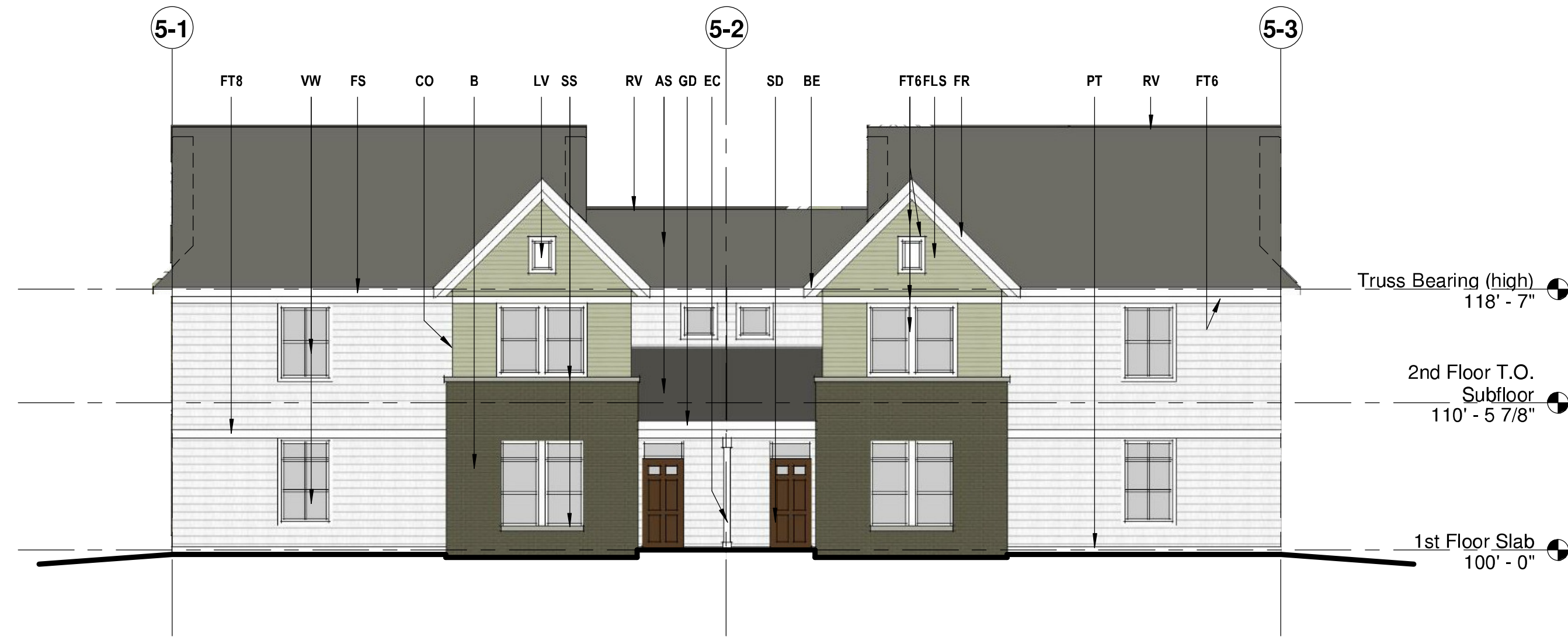
2 BUILDING TYPE E - SOUTH ELEVATION 1/8" = 1'-0"
