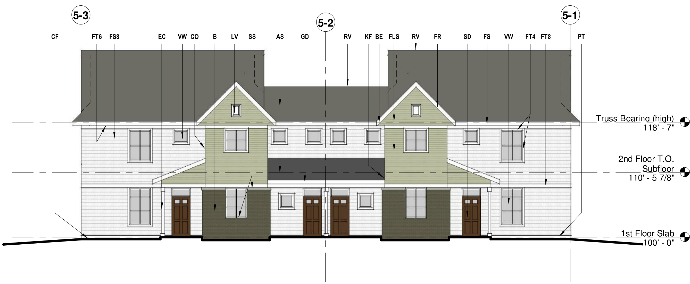
1 BUILDING TYPE E - NORTH ELEVATION 1/8" = 1'-0"
