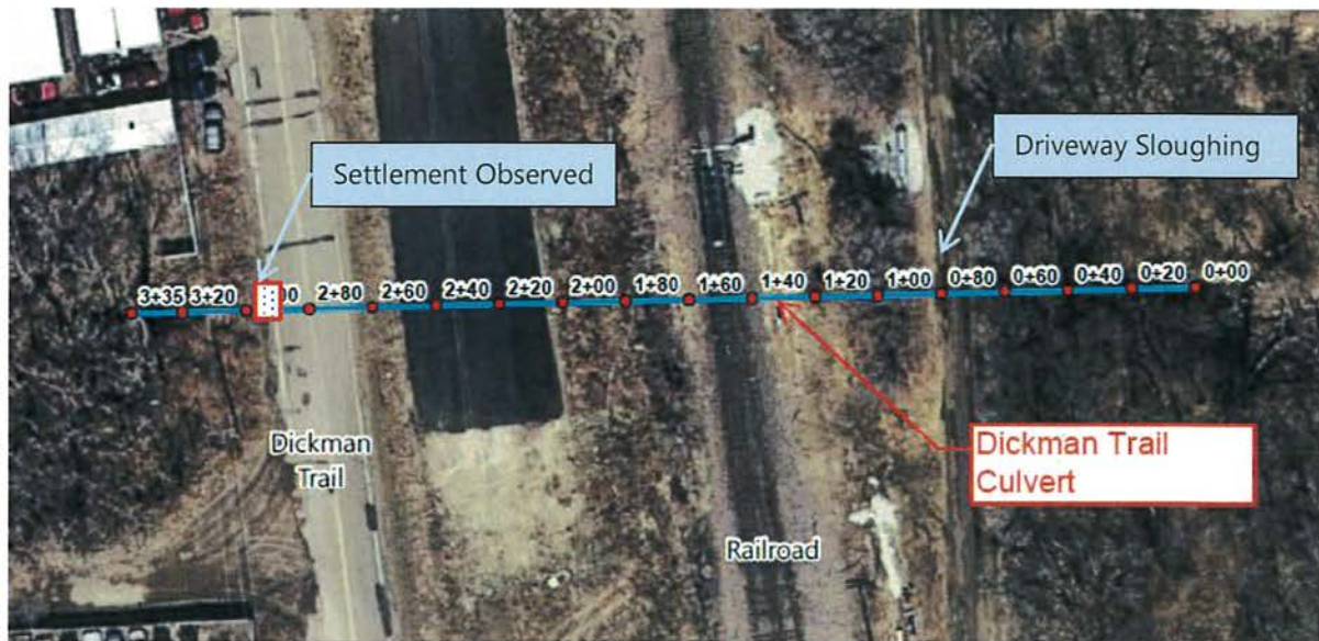
Figure 2-1 Dickman Trail Shoulder Settlement and Driveway Sloughing
