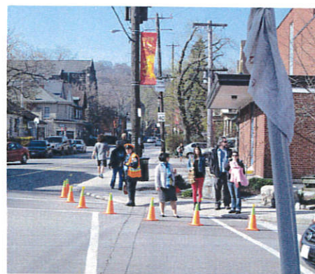
Tactical approaches to new facilities can be low-cost and temporary. The example above demonstrates how a temporary crosswalk bump out is being tested for future improvements
