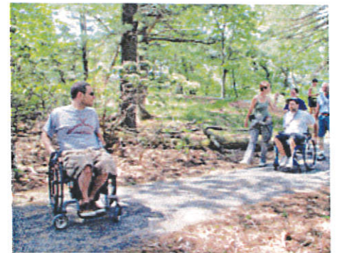
ADA accessible trails can be constructed with compacted gravel or asphalt surfaces, and maintain a low-slope
