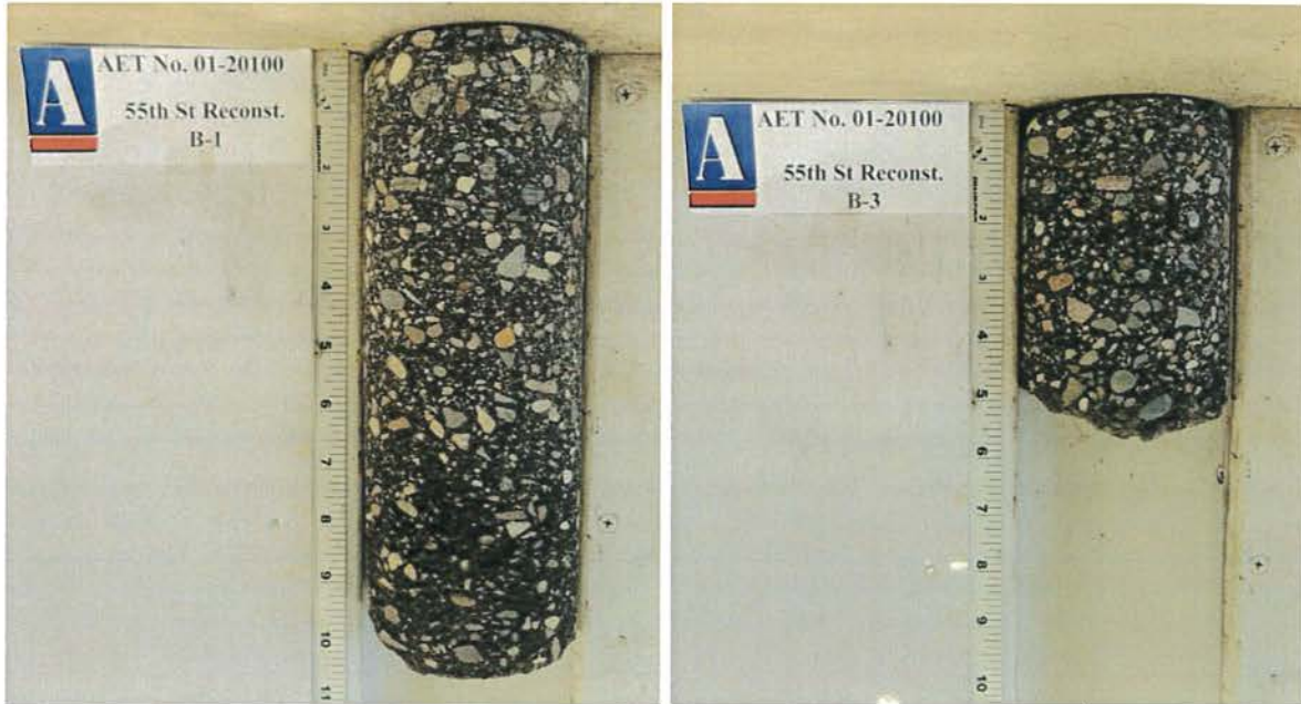
Figures 1a and 1b. Pavement cores offset from borings B-1 and B-3 on 55 th Street
