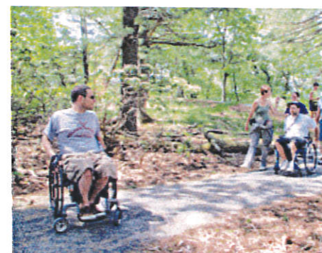
ADA accessible trails can be constructed with compacted gravel or asphalt surfaces, and maintain a low-slope
